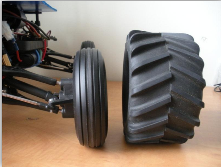
Figure 11: Du-Bro tire vs stock E-Maxx tire comparison
