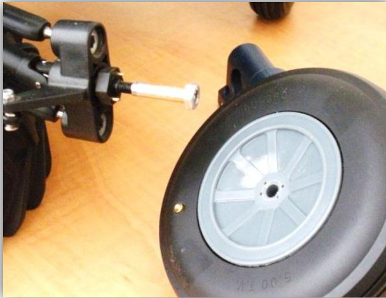
Figure 12: Modified E-Maxx wheel assembly
