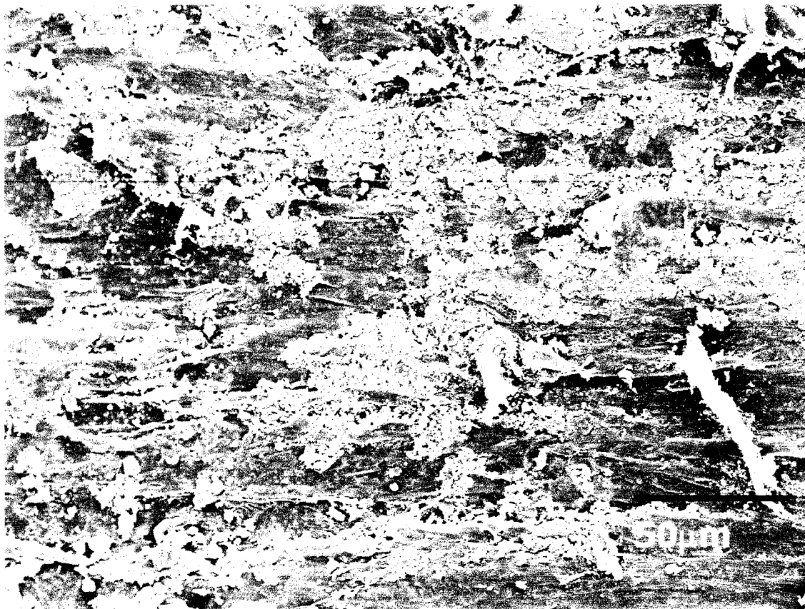
Fig. 4.17: Scanning Electron Microscopy of Delrin immersed in 100 mS/cm saline solution for 4200 h at 98 °C. Magnification, 500.
