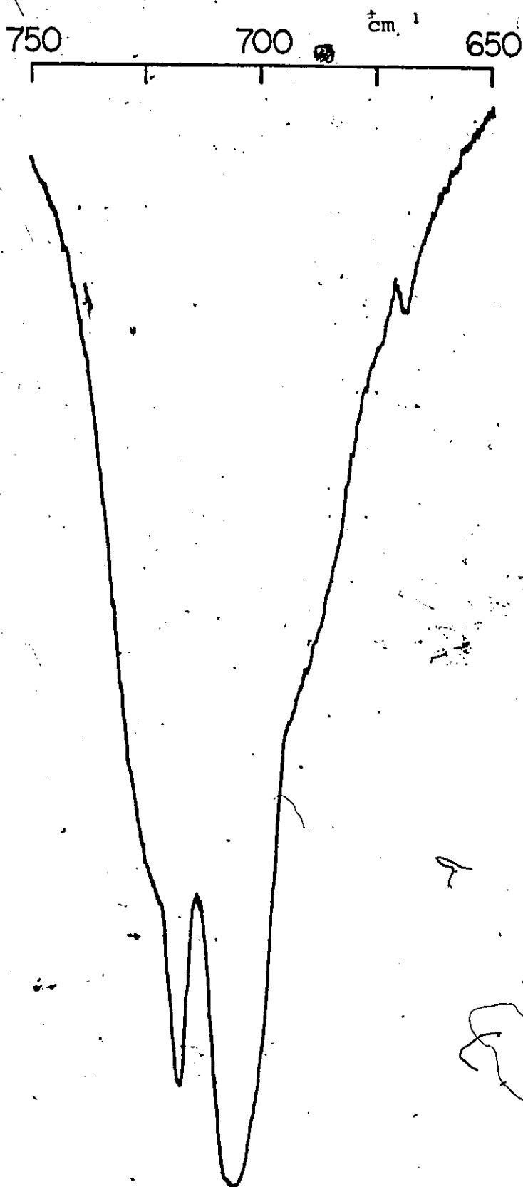
Figure I.1.6 Infrared spectrum (750-650 \text{cm}^{-1} ) of \text{CD}_3\text{SiD}_3
