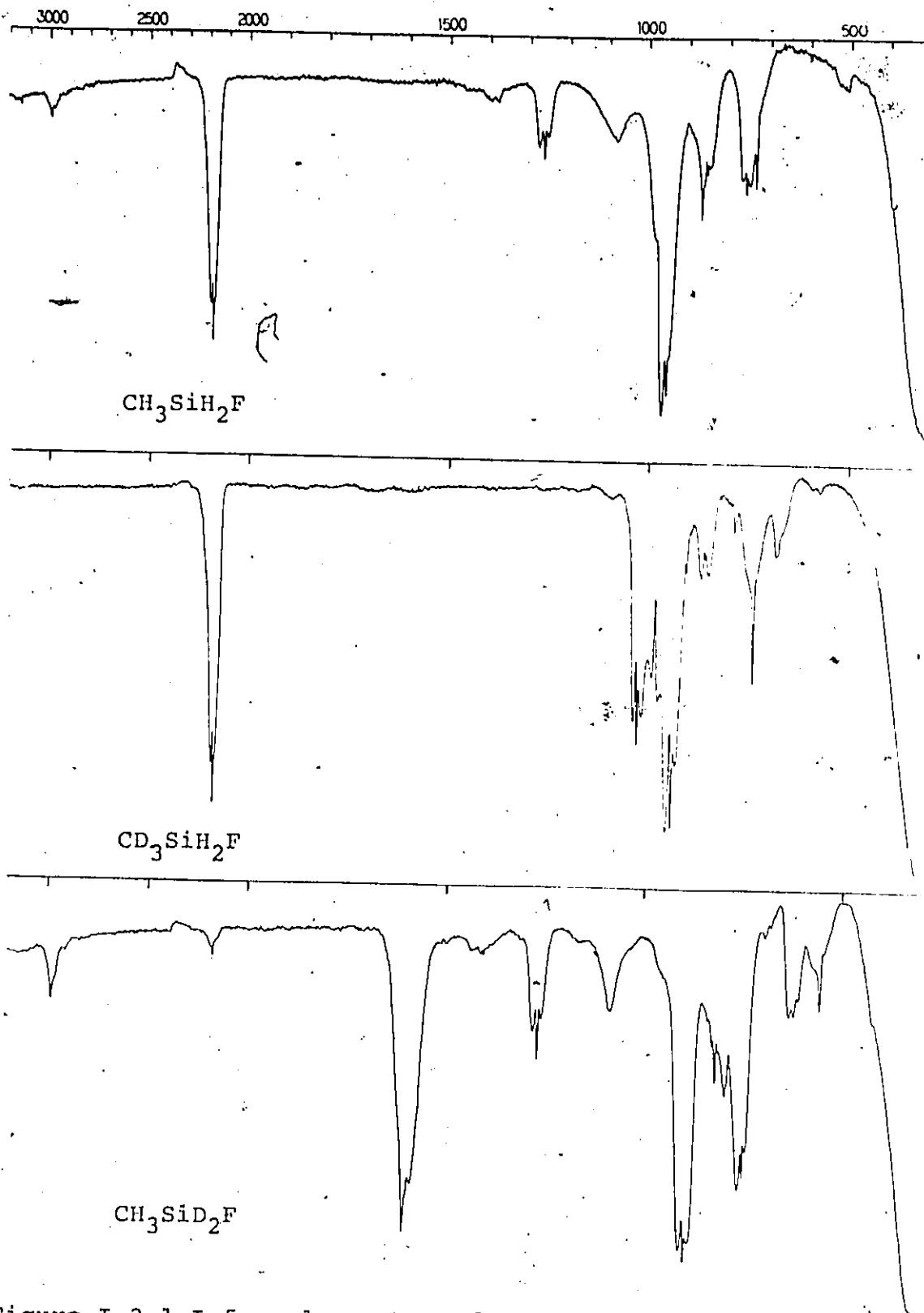
Figure I.3.1 Infrared spectra of the fluoromethylsilanes
