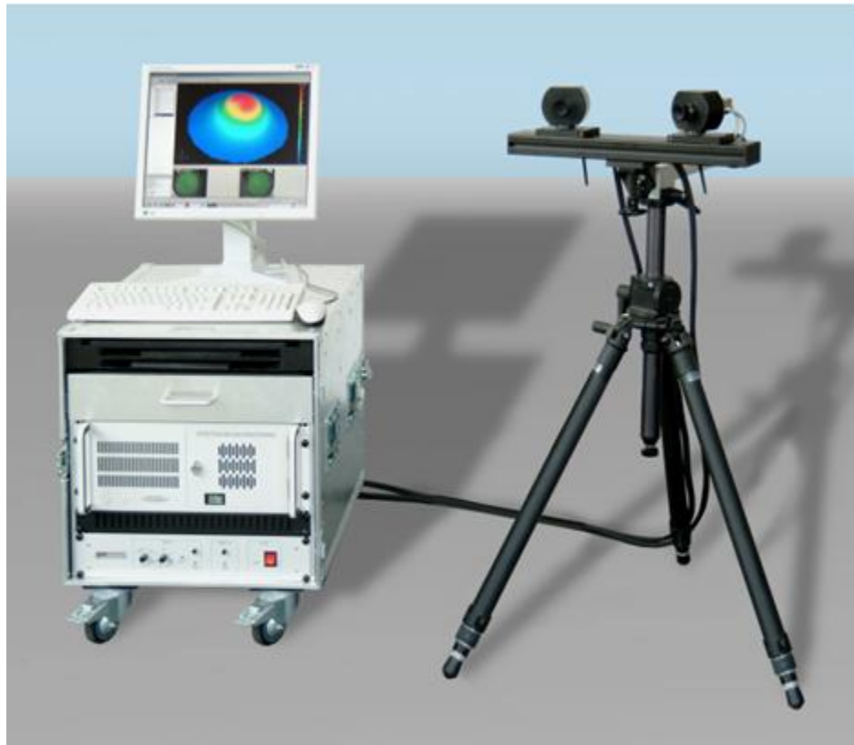
Figure 3.18: The hardware components of the ARAMIS DIC system (GOM mbH)
