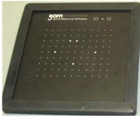
Figure 3.20: Calibration Panel (65 mm x 52 mm)
