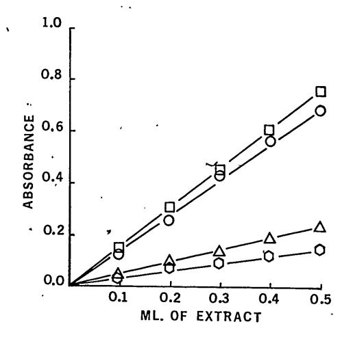
FIGURE 20. Oxidized chromogen formation as a function of the amount of crude <u>D</u>. <u>discoideum</u> myxamoebae trehalase extract. The experimental conditions for both continuous coupled and discontinuous assays were as described in the Materials and Methods section. The plotted values represent the absorbances of mixtures after correction for enzyme and substrate controls.
