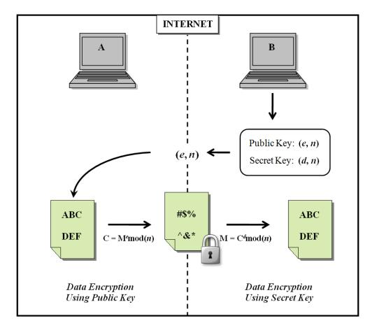
Figure 2.4: Data Encryption and Decryption Using RSA
