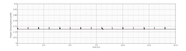
Figure 5.4: Power Consumption of two 32bit Digital to Analog Conversions (64 bits)
