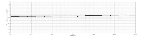
Figure 5.9: Power Consumption of two 32-bit Analog to Digital Conversions (64 bits)
