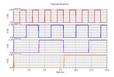
Figure 5.3: 4-bit Input B: Incrementing Value
