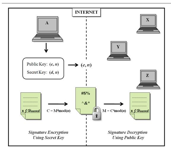
Figure 2.5: Signature Encryption and Decryption Using RSA
