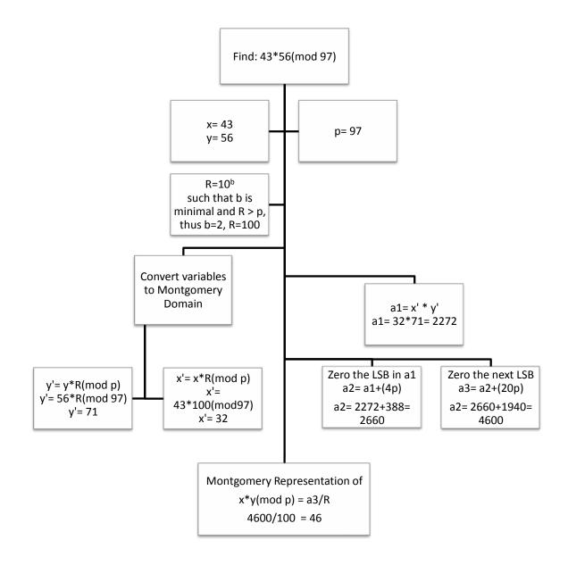
Figure 4.1: Modular Multiplication Using Montgomery Method
