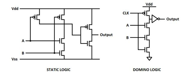
Figure 5.5: Static versus Dynamic Logic
