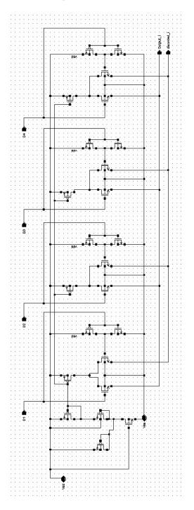
Figure 5.1: Transistor Level Diagram of One a One Bit Conversion
