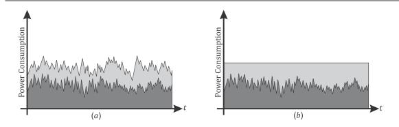
Figure 3.1: Countermeasure Techniques: (a)Masking (b)Hiding
