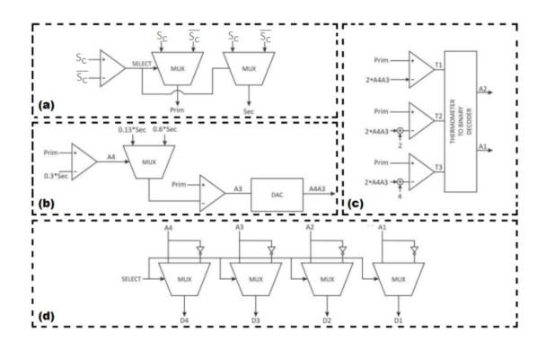
Figure 4.7: Block Diagram of Proposed ADC Design
