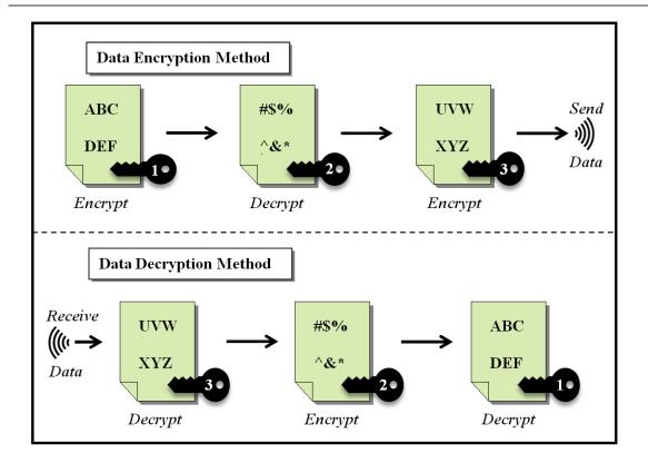
Figure 2.2: Encryption and Decryption using 3DES
