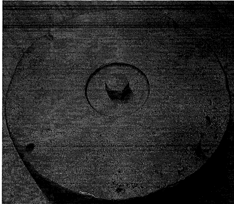
Figure 3.4 Squeeze cast cylindrical coupons with dimensions of approximately 100 mm in diameter and 25 mm in thickness.
