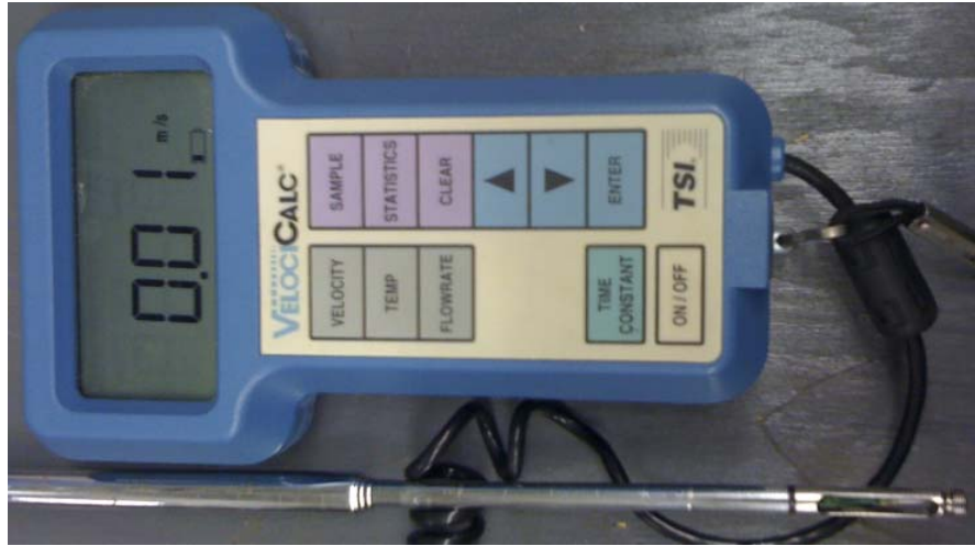
Figure 4.18. Handheld digital hot-wire anemometer (HWA) – backup air velocity measurement.
