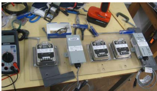
q. Airside Pressure Transducers Panel Making
