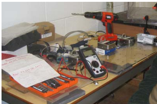
o. Airside Pressure Transducers Testing
