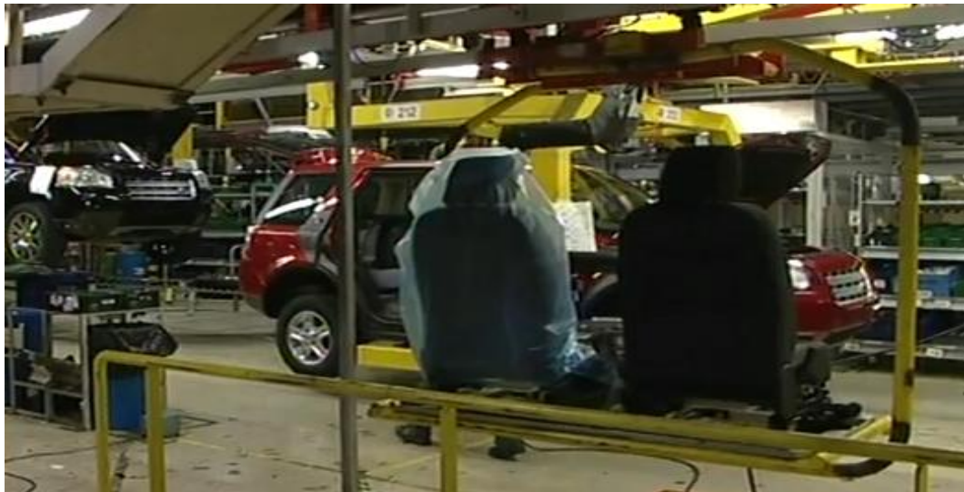
Fig. 2- 9: Car body at final assembly (seat installation) (GM, Lancing)
