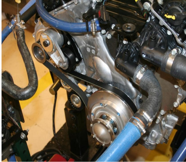
Figure 3.7 - Picture of the start cart BSG system.
