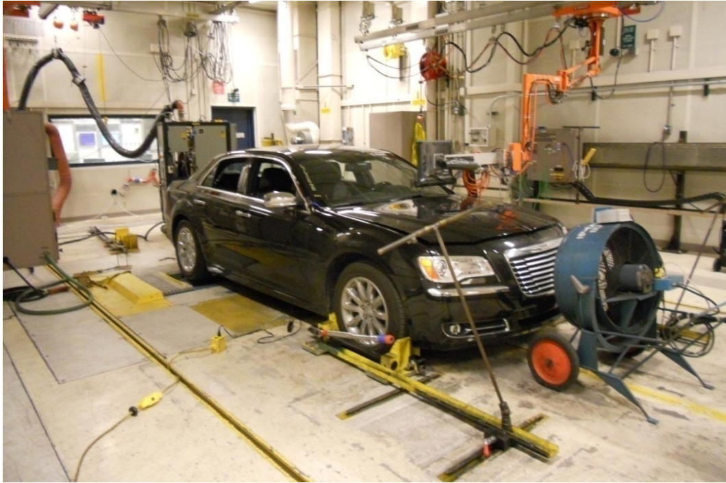
Figure 3.47 - Proof-of-concept test car on the dynamometer. The screen over the windshield shows the speed profile of the cycle.
