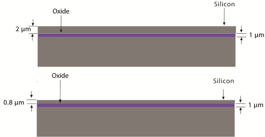
Figure 5-4 Step 1: Thinning SOI Wafer
