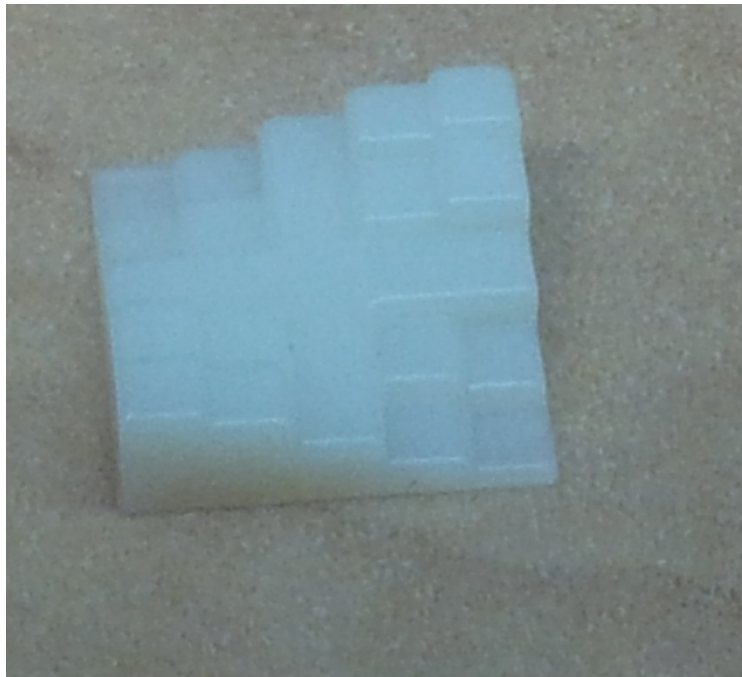
Figure 5-19 Verowhite plus Fullcure835 3D printed non-planar array
