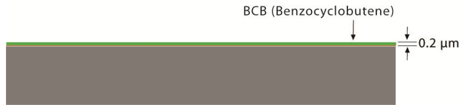
Figure 5-10 BCB coating (200 nm)
