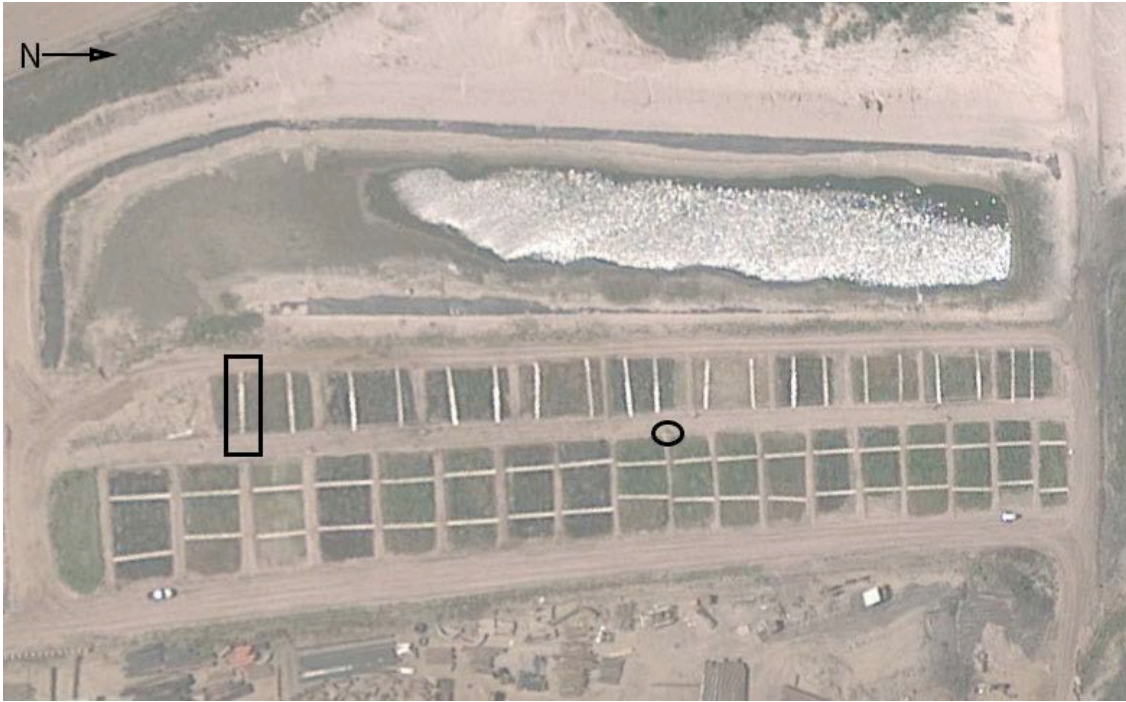
Figure 2.2: Aerial photo of experimental field. Circle indicates position of meteorological station. Rectangle indicates a cell boardwalk (2 boardwalks in each 10 x 20 m cell). Note the white pickup truck in the lower left corner for scale.
