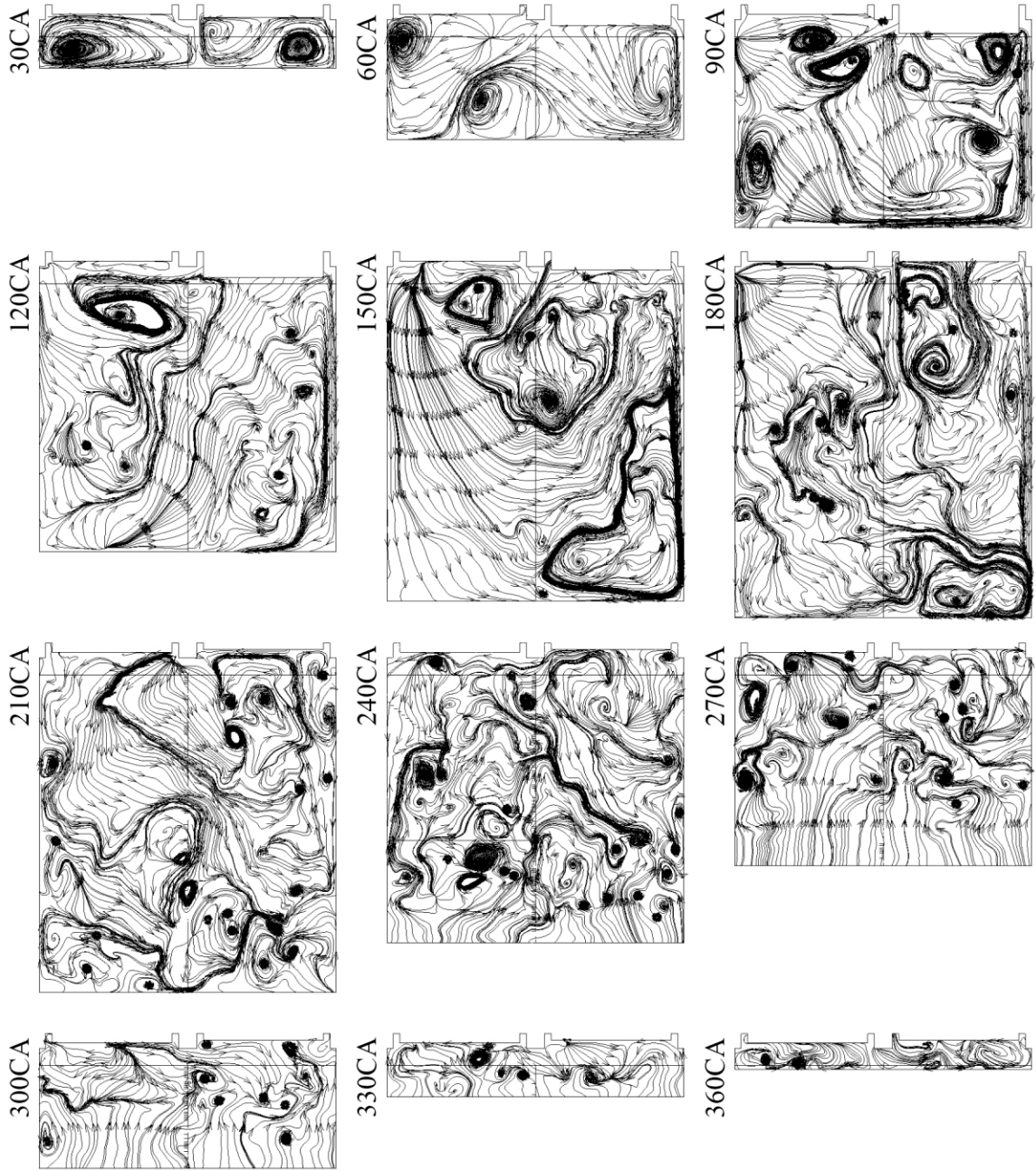
Figure A.8 – Naturally aspirated in-cylinder flow structure development by the DES Spalart-Allmaras model with fine mesh
