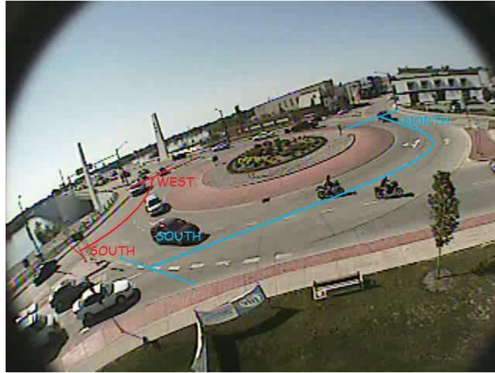
Figure 4-4. Example of Path for Estimation of Free-flow Speed.
