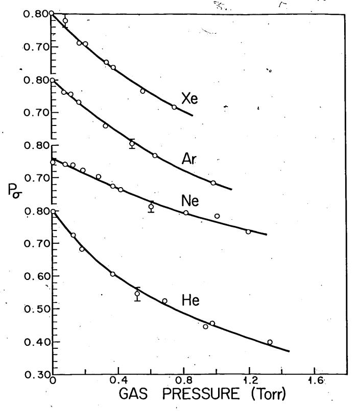
Figure 22. Variation of the degree of linear polarization of the 8521-A resonance fluorescence with noble gas pressure at zero field.
