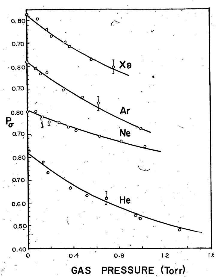
Figure 20. Variation of the degree of circular polarization of the 8521-A resonance fluorescence with noble gas pressure at 5.3 kG.
