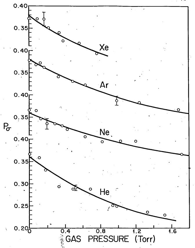
Figure 18. Variation of the degree of circular polarization of the 8521-A resonance fluorescence with noble gas pressure at 0.6 kG.
