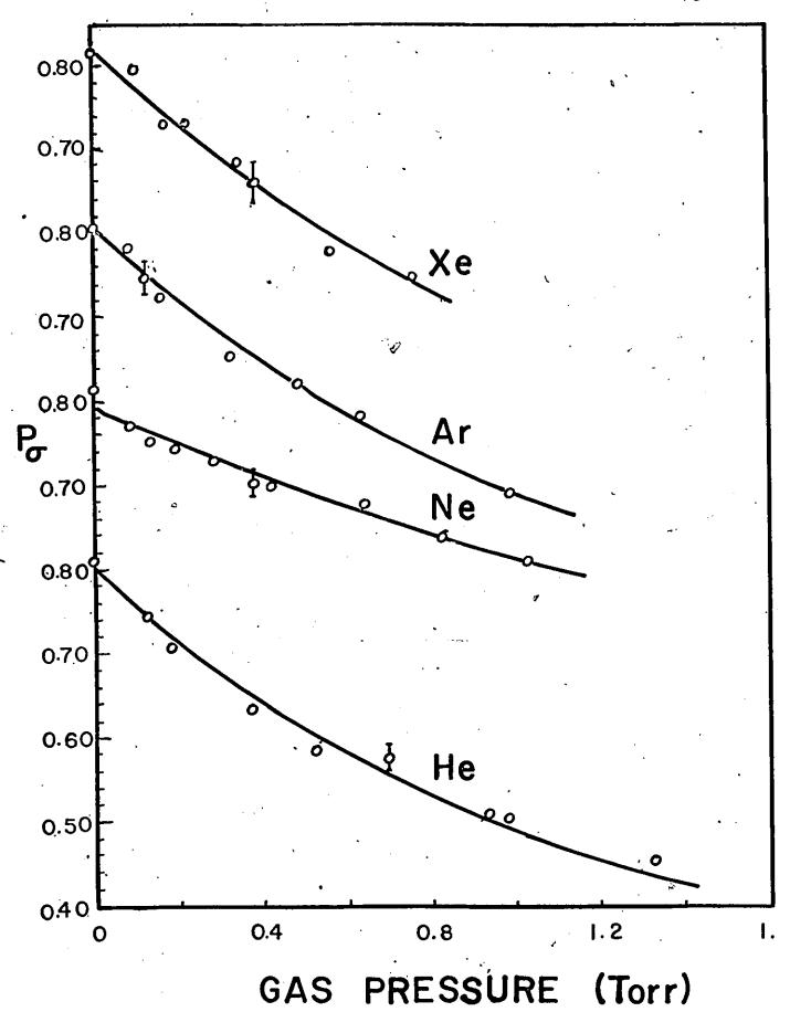
Figure 21. Variation of the degree of circular polarization of the  $8521-\mbox{\ensuremath{\mbox{A}}}$  resonance fluorescence with noble gas pressure at 6.7 kG.
