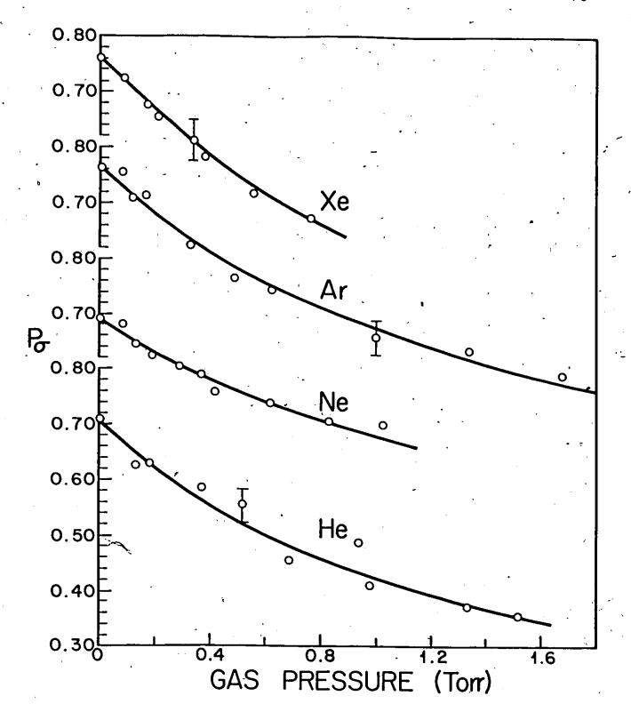
Figure 19. Variation of the degrees of circular polarization of the  $8521-\text{\AA}$  resonance fluorescence with noble gas pressure at 3.8 kG.
