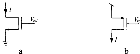
Figure 3.5 Schematic of current sources: (a) nMOS current source, (b) pMOS current source.
