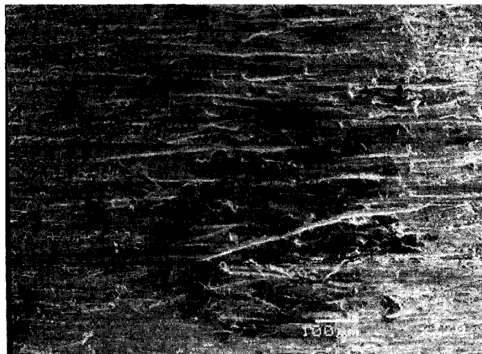
Figure 5.20 Worn surface of the M2 counterface against A13-C-T6 specimen (x100). Small amount of transferred aluminum and debris attached on the scuffed counterface.
