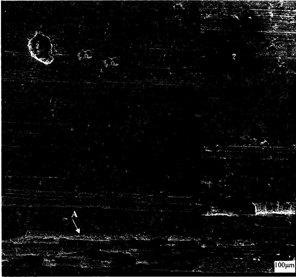
Figure 5.19 Scuffed surface of the A13-C-T6 specimen. Area marked A shows deep galling occurred on the surface.
