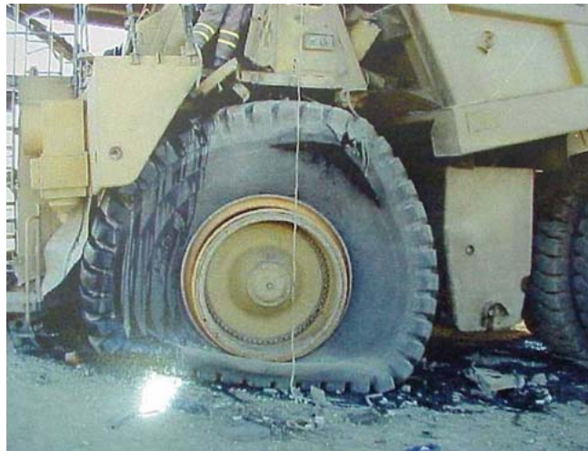
Figure 2.3.1 – Result of tire zipper failure [21].
