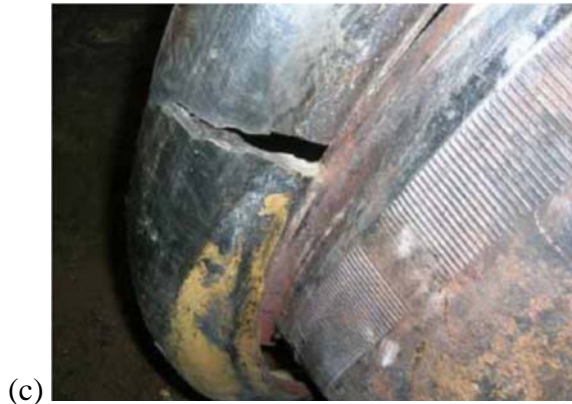
Figure 2.3.2 - Photos of failed wheels illustrating (a) tire damage due to flange separation, (b) rim base wear and fatigue crack, and (c) a cracked outer flange [21].
