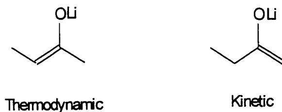
Figure 10. Thermodynamic versus kinetic enolate
