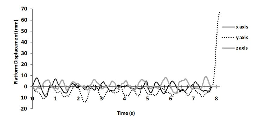
Figure 10. An example of the robotic platform displacements in each of the axes for the perturbation protocol in the back direction condition that the vibration group subjects experienced. Note that this is an example of vibration occurring from the beginning of the trial up to 7.75 seconds which is followed by the perturbation in the y axis.
