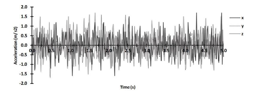
Figure 9. A graphical representation of the acceleration profiles for each axis that were used to create the robotic platform motions, which were experienced by participants in the vibration group. The average RMS acceleration in each of the axes was  $0.55 \text{m/s}^2$ .
