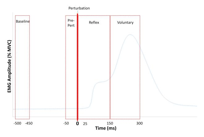
Figure 15. The four time periods are shown relative to the time profile of the perturbation (blue line).
