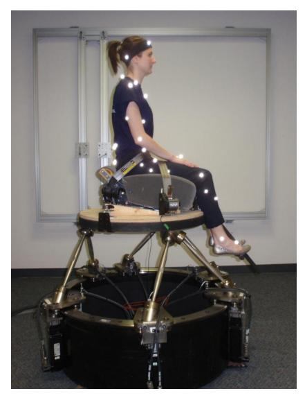
Figure 14. Participants were seated on a backless car seat and told to maintain neutral posture during both the pre-perturbation and perturbation protocols.
