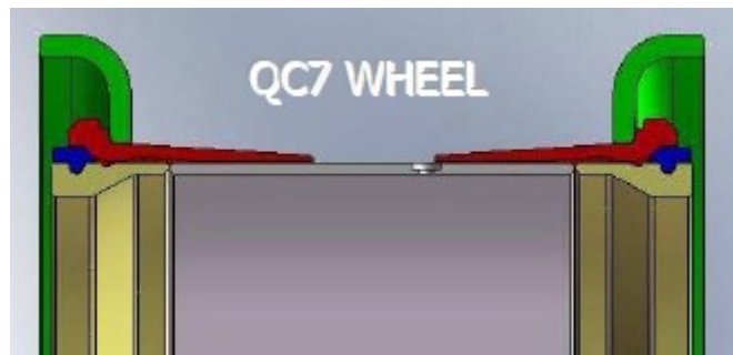
Figure 2.7 The structure of a seven-piece wheel [22].
