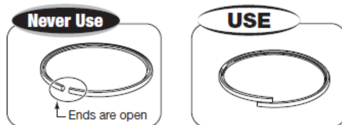
Figure 2.14 A sprung lock ring (left) and a good lock ring (right) [18].
