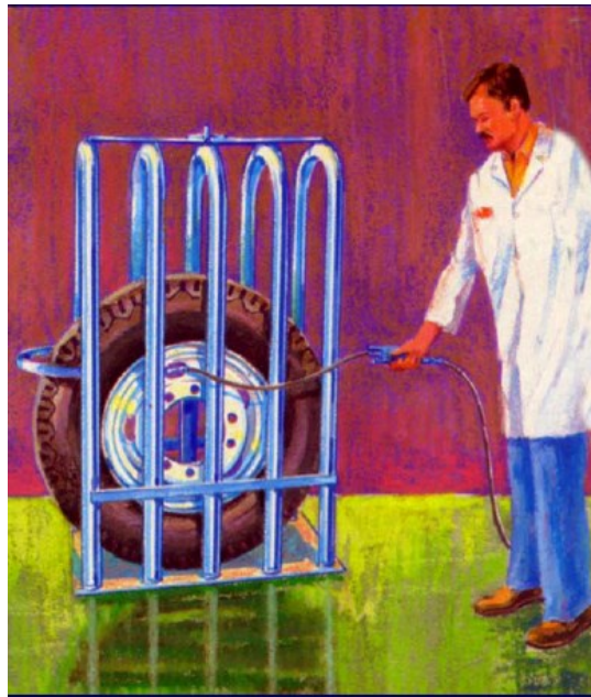
Figure 1.8 Wheel and tire in a safety cage during tire inflation [11].
