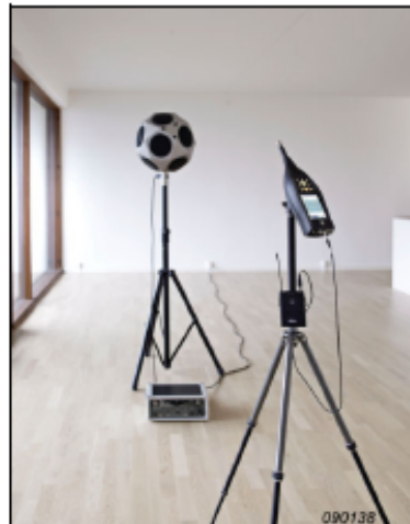
Fig. 21 Reverberation Time measurement – measured using the interrupted noise method
