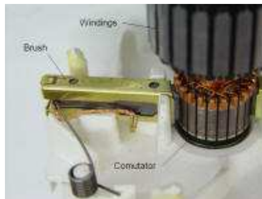
Figure C.1. DC commutator and brush
