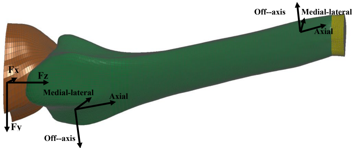
Figure 4.11: Model Accelerometer Locations
