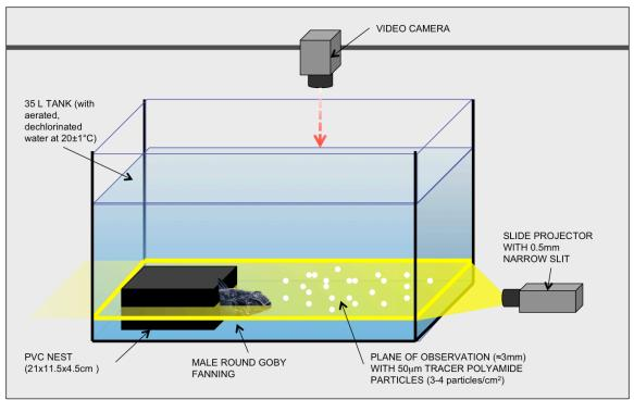
FIG. 1: PIV image analysis setup.
