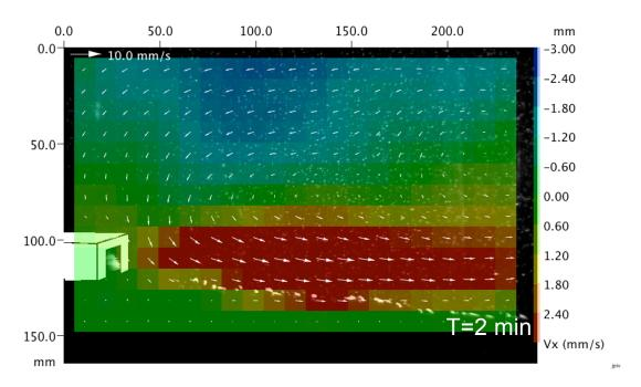
**FIG. 3:** Vertical flow visualization: Time-averaged velocity field during a caudal fanning bout. The nest entrance is on the left side of each diagram. The scale of the coordinate system is 1 pixel/0.343 mm (top and left axis). The temporal resolution is 0.04 s (25 frames per sec). T is the duration of the fanning bout. The color code represents the time-averaged velocity of the particles in the X dimension.
