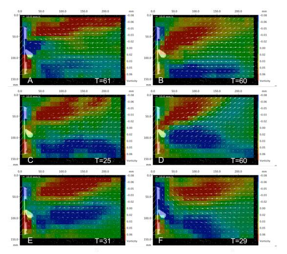
**FIG. 4:** Horizontal flow visualization: Time-averaged vorticity fields for 6 different caudal fanning bouts. The nest entry is on the left side of each diagram. The scale of the coordinate system is 1 pixel/0.343 mm (top and left axis). The temporal resolution is 0.04 s (25 frames per sec). T is the duration of the fanning bout in seconds. The color code represents the orthogonal vorticity of the flow.
