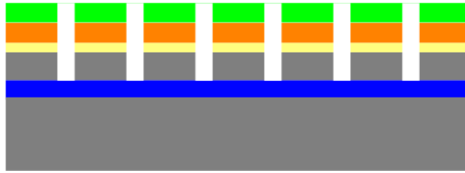
Figure 4.9. Silicon DRIE etch.
