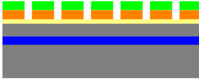
Figure 4.7. Metal and silicon etch.
