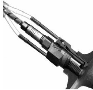
Figure 4.9: Kistler Pressure Transducer Assembly (Taken from [19])
