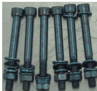
Figure B.24: M8 Main Flange Bolts
