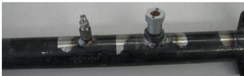
Figure 4.6: Modified I-TEC Exhaust Pipe
