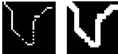
Figure 4.7: Edge enhancement property of the Maximum filter. The right image is the result of applying Maximum filter on the left image
