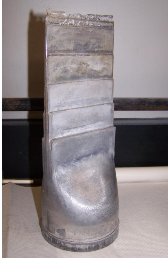
Figure 3- 3. A 5-step casting solidifying under applied pressure 30MPa.
