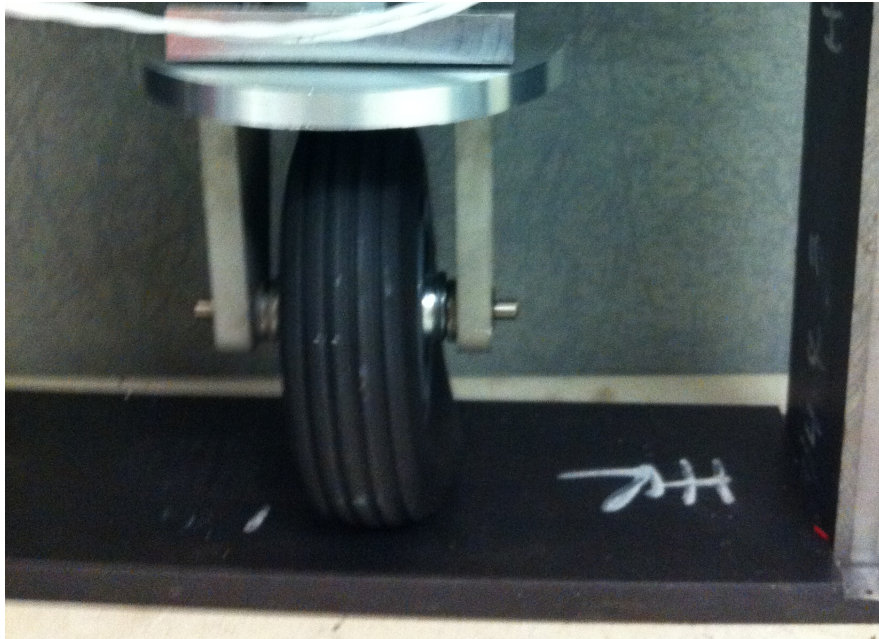
Figure 5.12: DUBRO 5.00 T.V. residual tire deflection with full removal of lateral load during 70 N normal load test.
