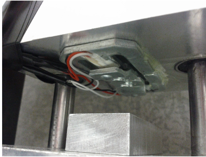
Figure 4.3: WATT vertical load sensing block . The two load cells in the figure are placed in line with the load placed by the drive screw, allowing direct measurement of the applied vertical tire load.
