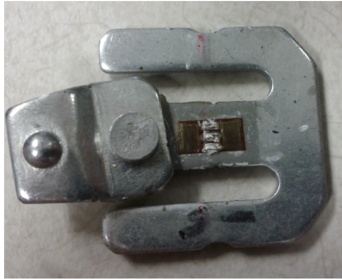
Figure 4.6: WATT internal construction of the load cells. Each cell features two active strain gauges oriented on the top surface.
