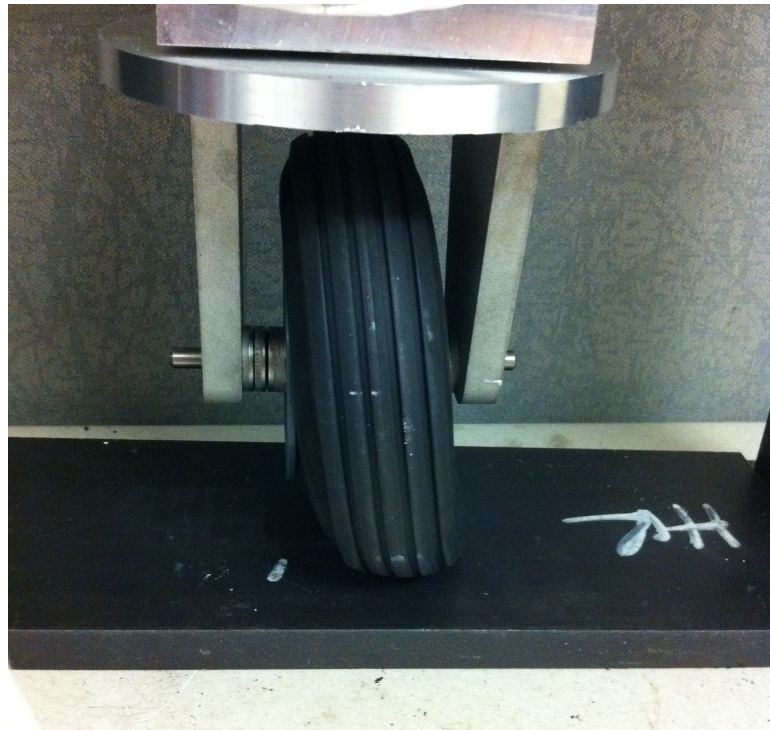
Figure 5.10: DUBRO 5.00 T.V. tire wheel separation at large deflection under 70 N normal load.
