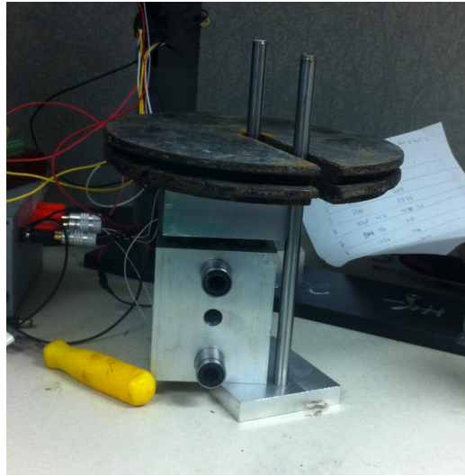
Figure 4.14: Lateral axis load cell calibration set-up. Due to the four posts present in the lateral axis, a single post of the vertical axis carrier block was utilized to support the lateral load sensing block during calibration.
