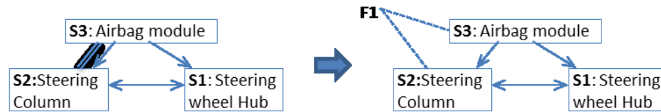
Figure 5.9: Substance-Field formulation for airbag joint
