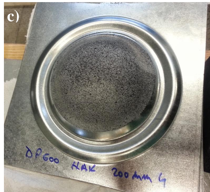
Figure 3.3: a) Nakazima test setup; b) hemispherical punch; c) formed specimen showing the DIC speckled pattern.
