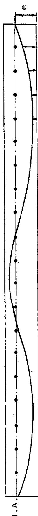
FIGURE 6.9 WIRE PROFILE AND ECCENTRICITIES OF THE CURVED TENDONS FOR SKEW SLAB PC4 (in mm)
