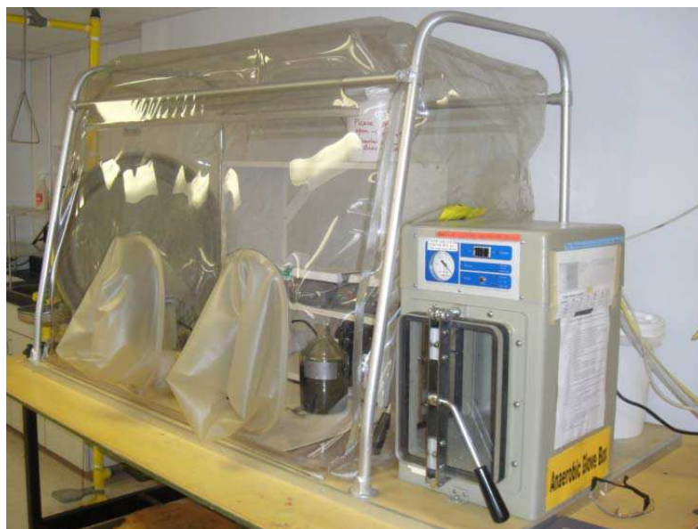
Figure 3.2: Coy® anaerobic chamber
