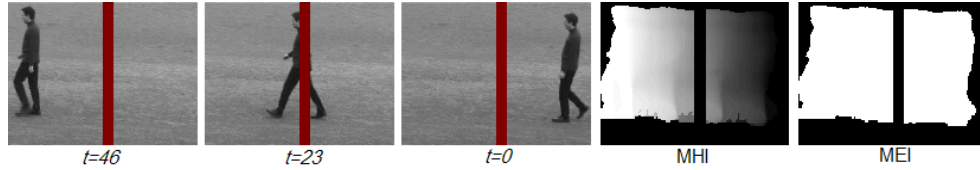
Figure 2.5: Temporal templates. From left to right: three key frames of a video clip of a walking actor showing a hand-made occlusion (the vertical red bar), and motion history and energy images of the same motion. They show no tolerance against the effect of temporal occlusion.
