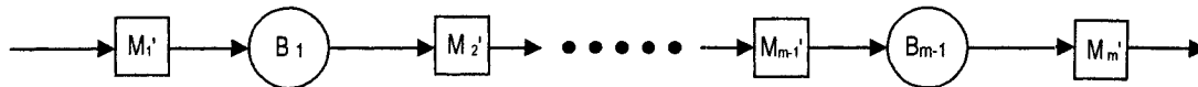
Figure 4.5: Serial flow line (replacing each set of parallel machines by an equivalent machine)
