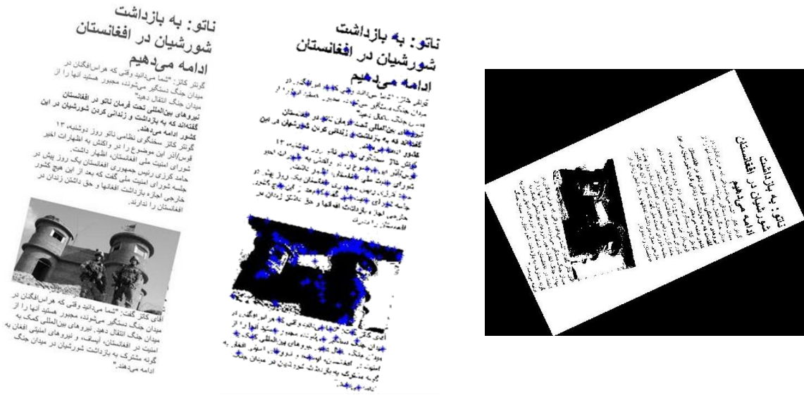
Figure 13: A skewed image of a page (left), connected components used for N-N skew detection method (middle), incorrect skew correction (right)
