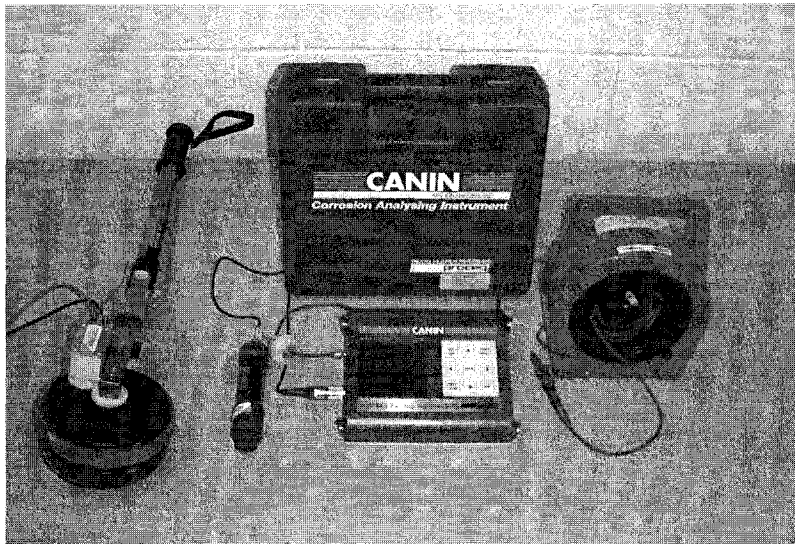
Fig. 4.23 CANNIN half-cell equipment with rod and wheel electrodes
