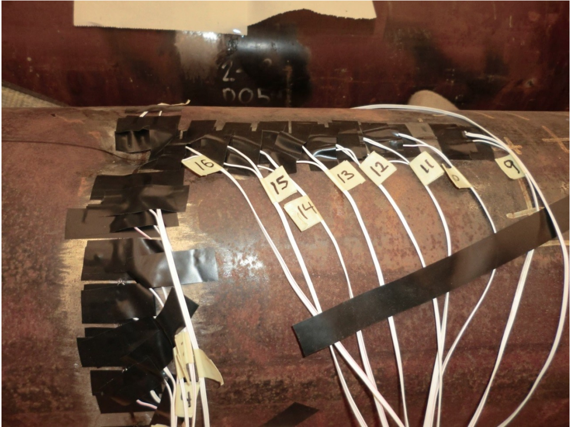
Figure 3.6: Photo of Strain Gauge Locations for Sphere and Dome Indented Pipes
