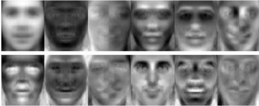
Figure 3.5: Samples of eigenface images: The mean image of facial images at the top left corner, followed by the top eleven eigenfaces.
