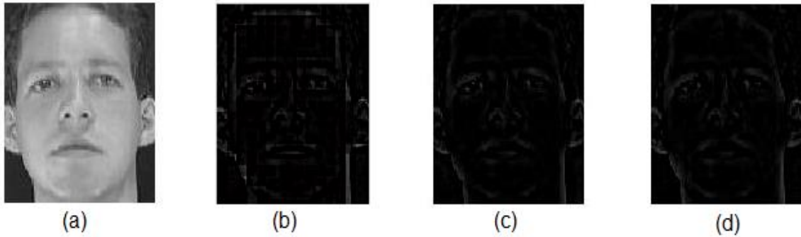
Figure 2.9: Interpolation error. (a) the original image. (b) the difference image between (a) and the reconstructed image using nearest neighbor. (c) using bilinear interpolation. (d) using bicubic.
