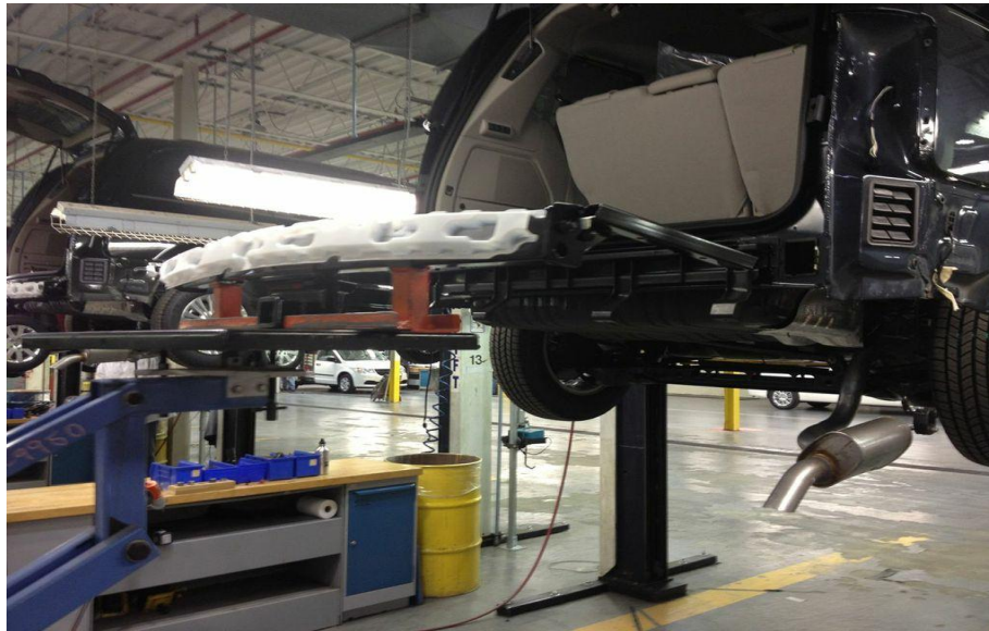
FIGURE 3- 8 SLIDE THE HITCH RECEIVER INTO THE FRAME RAILS
