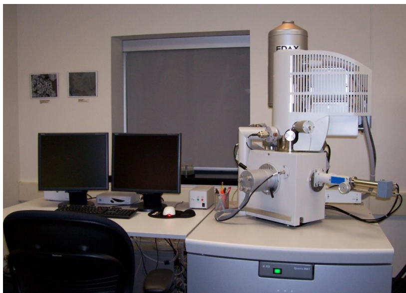
Figure 2.4. FEI Quanta 200 Environmental scanning electron microscope. This was the instrument employed in all the SEM work for this thesis. Image courtesy of Mrs. Sharon Lackie
