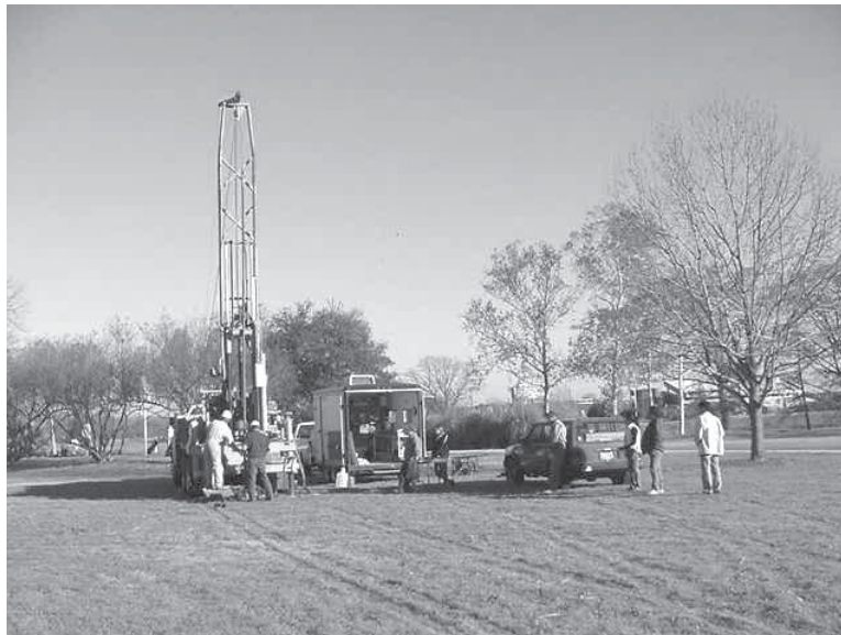
Figure 5-6. Core drilling on the edge of the Golf Course between Spring Lake and Sink Creek.
