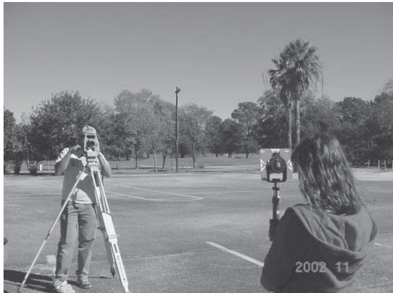
Figure 5-1. Excavation units and bore holes were mapped using a Sokkia total data station.
