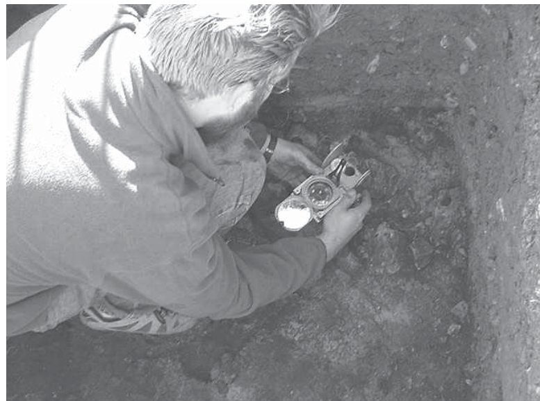
Figure 5-4. After drilling a core in the fire-cracked rocks, measurements were taken using a brunton compass mounted on a goniometer.
