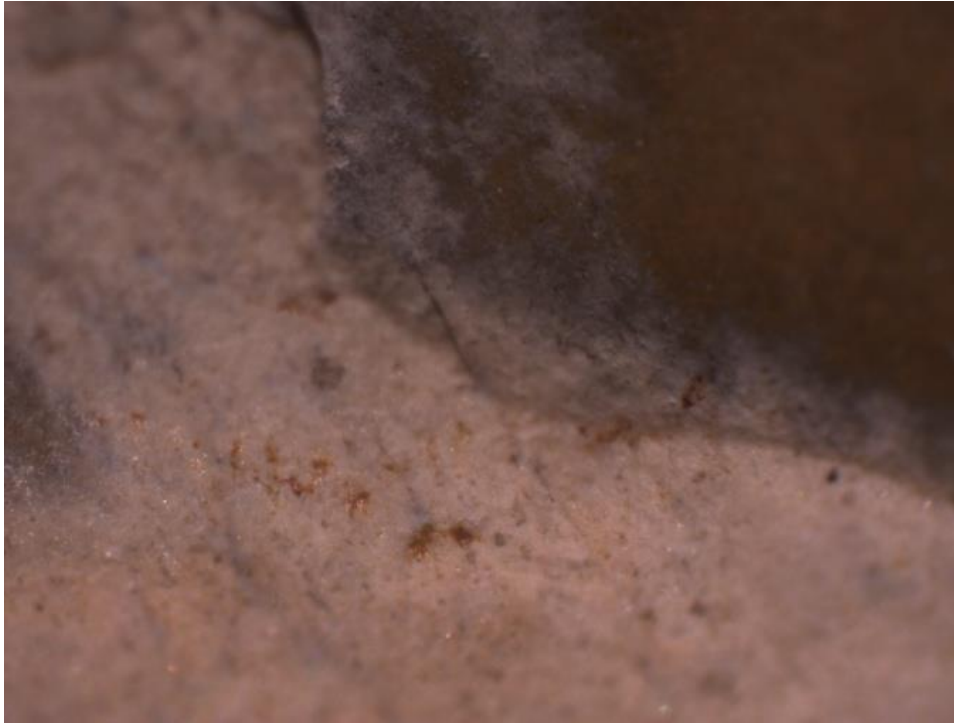
Figure C-7. Specimen P1724: rust spots on the body of specimen.
