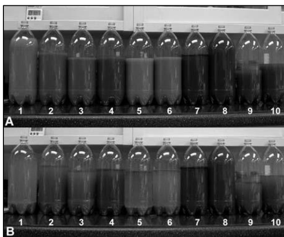
Figure F-5. Decanted sample solutions containing silt and clay after decanting from the sand fraction.
