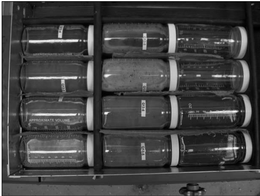
Figure F-2. Samples in Calgon® solution on mechanical reciprocal shaker which was set at 180 strokes/- minute. The samples were shaken vigorously for 24 hours. The two empty jars in the upper right corner served as spacers (2-27-13).
