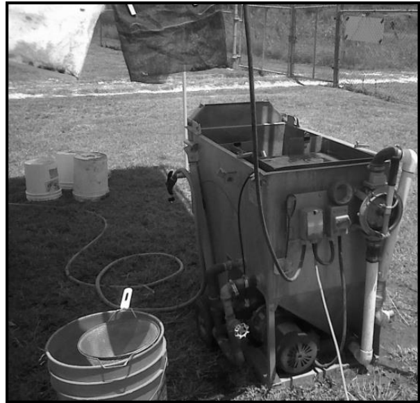
Figure 4-4. Dousman flotation system used to float sediment samples.
