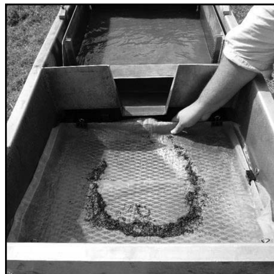
Figure 5-9. Dousman flotation system employed to float sediment samples (light fraction in tray).
