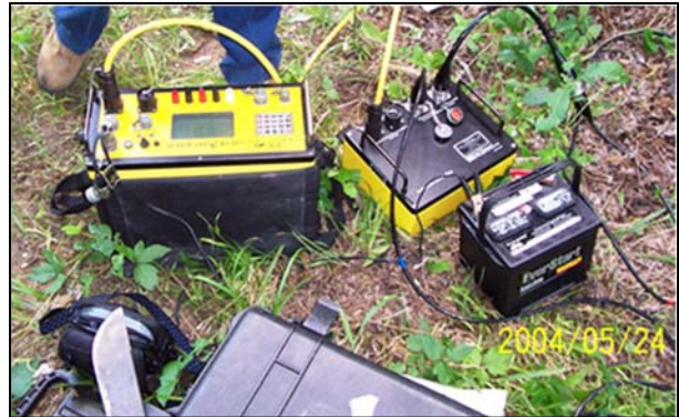
Figure 4-1. Electrical resistivity equipment employed in the geophysical study.
