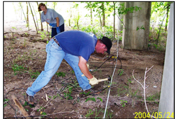
Figure 4-2. Setting resistivity probes at 1 m intervals in APE.
