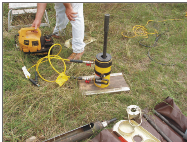
Figure 4-4. Hydraulic lift being used to extract the gouge from Core #2.
