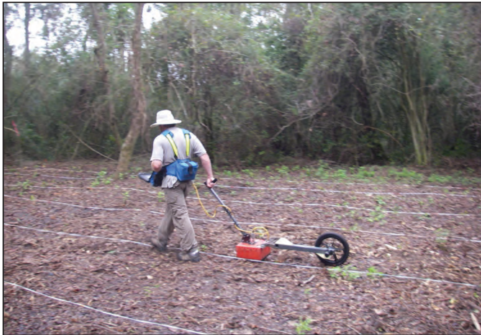
Figure 7-12. The GSSI SIR2000 GPR with the 400-MHz antenna operating in the small cleared area north of the Broussard Cemetery.
