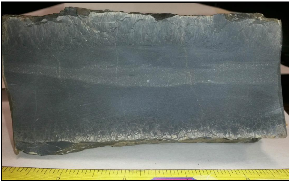
Cross section view showing crust and core, and conal structures. Scale in inches.
