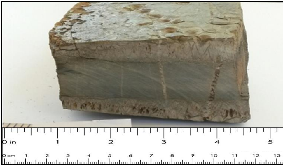
Figure 8. Clearly defined interior and exterior boundaries with grossly visible cone structures in the exterior
