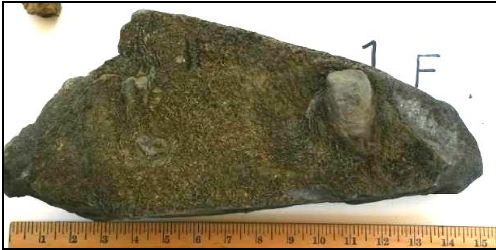
Top view showing cone shells and clay cone fillers clearly distinguishable; cone shells growing into clay layers. Scale in inches.
