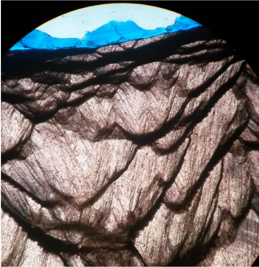
Upper shale crust with underlying slightly larger cones than interior cones (40x)
