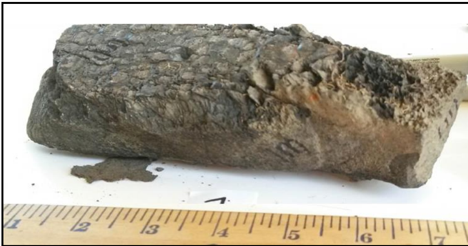
Top and side view; scaly top crust. Scale in inches.
