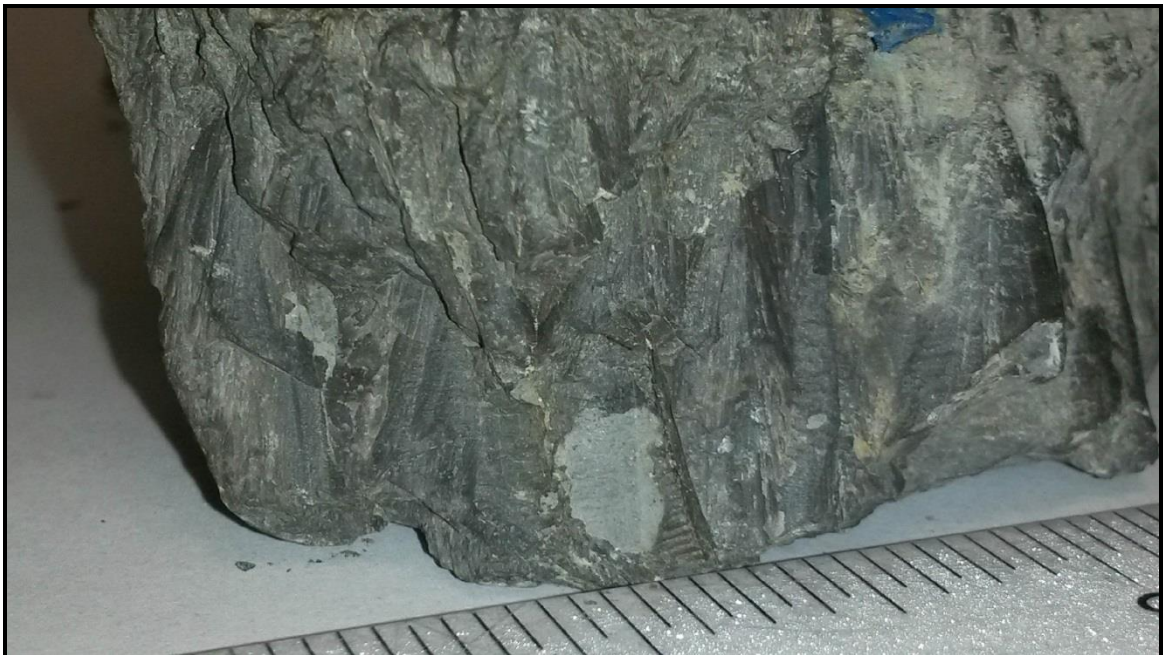
Close up view of cone in cone structures. Scale is inches.
