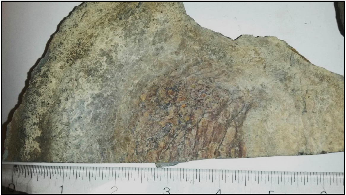
Scaly appearance of bounding surfaces. Scale in inches.
