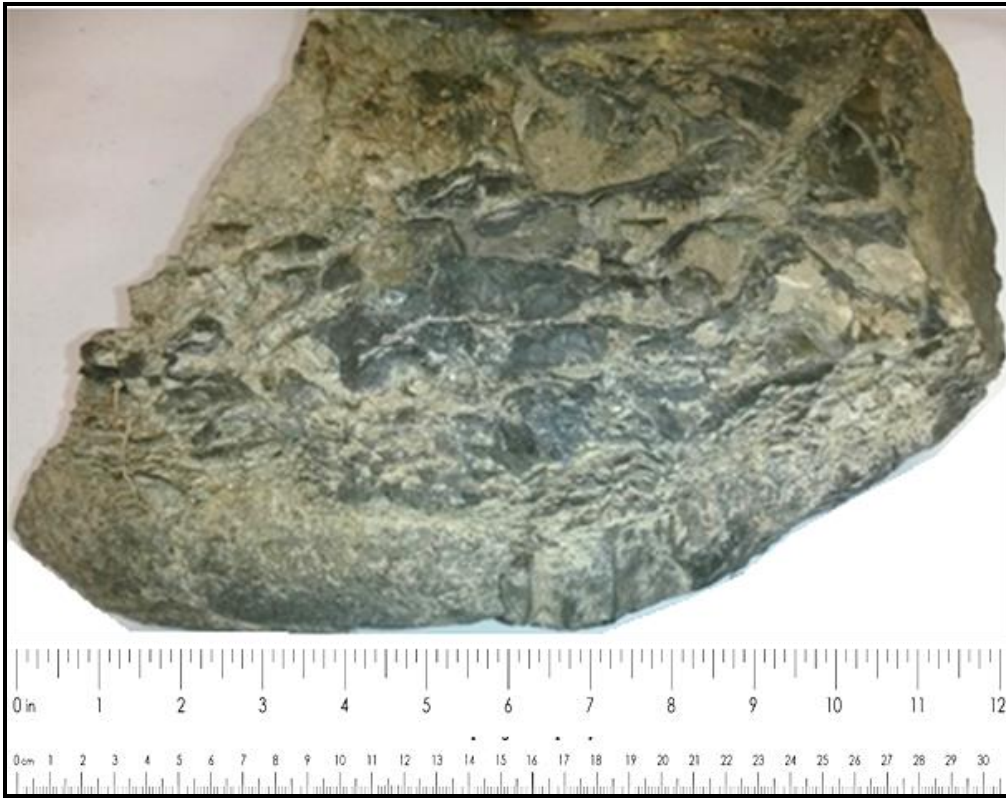
Top view with irregular conal shapes, high degree of weathering
