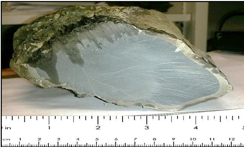
Cross section view showing wedge shaped bottom and side crust. Epoxy infiltration permeated through cone shells and fillers indicating pathways for fluid movement both inward and outward. Scale in inches and centimeters.
