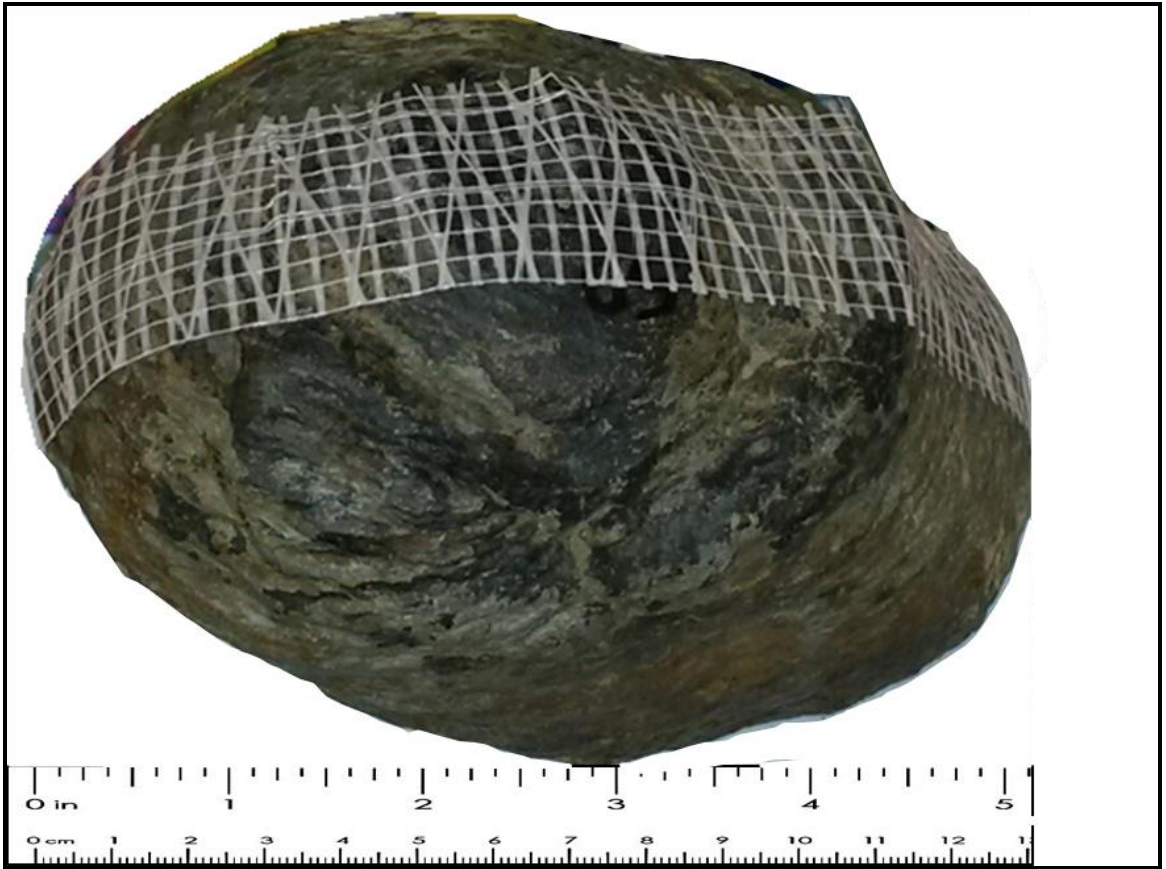
Top view of horned concretion with layering slightly evident in picture. Sample has been epoxied and ready to cross section.
