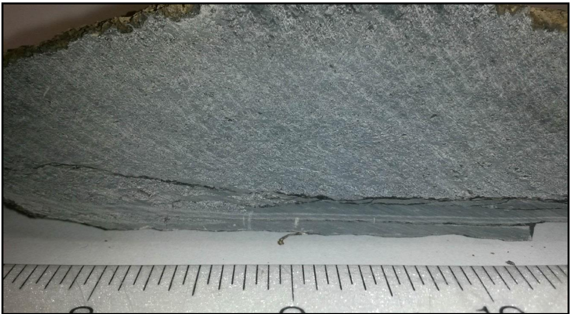
Bottom view of cross section: Shale layer with microscopic cone structures just above. Scale in inches.
