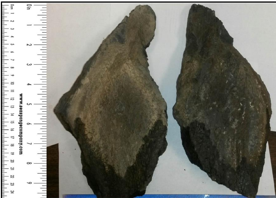
Top view looking down at the two fractured pieces that fit on top of each other with scaly appearance.
