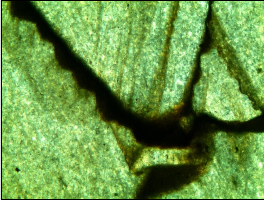
Apex of large upper crust cone shell and annular rings (100x)
