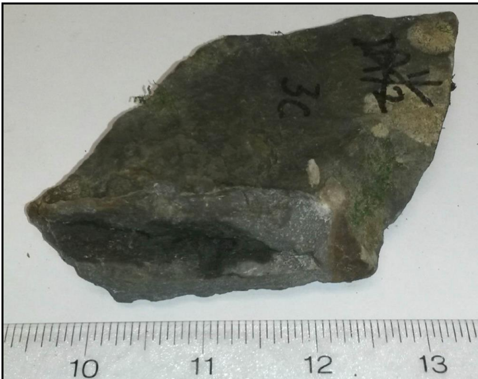
Side view showing carbonate rich shale in the core center. Scale in inches.
