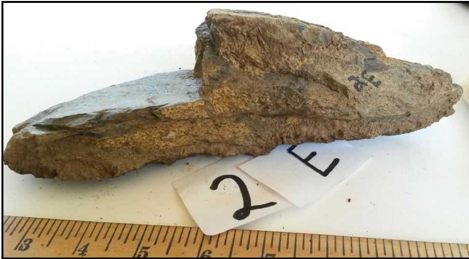
Side view showing light colored core with vuggy appearance, and multiple layers of visible cone structures. Scale in inches.
