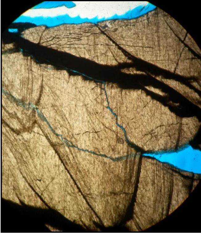
Exterior cone and cone shells with annular rings, twinned lamellae calcite (40x)
