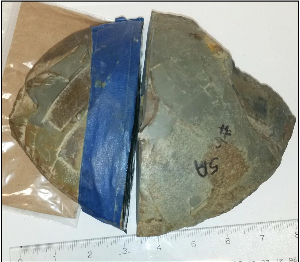
Top view of concretion after cross sectioning, notice the smooth outer shale surface. Scale in inches.
