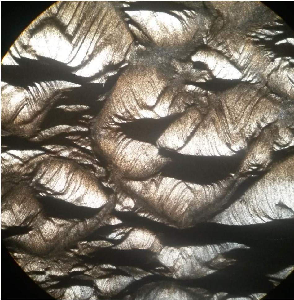
Figure 20. Opposing cones with lenticular banding and clay lineations, mostly perpendicular to cone shells. (100x).
