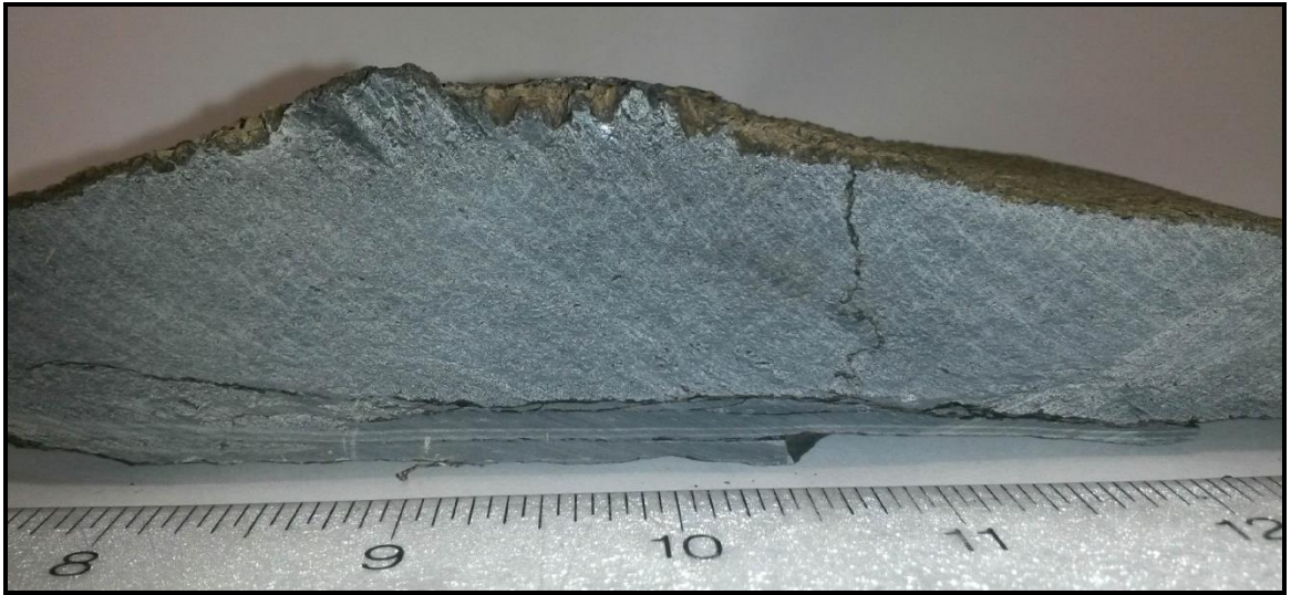
Cross section with bounding shale layer along the bottom. Scale in inches.
