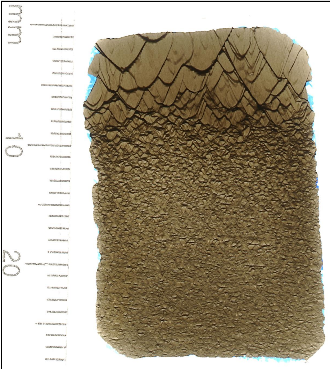
Thin section gross photo. Sample 1D top of concrete. Top of concrete or upper crust is at top. Cone in cone structures seen throughout. Large cones only seen on the upper crust.
