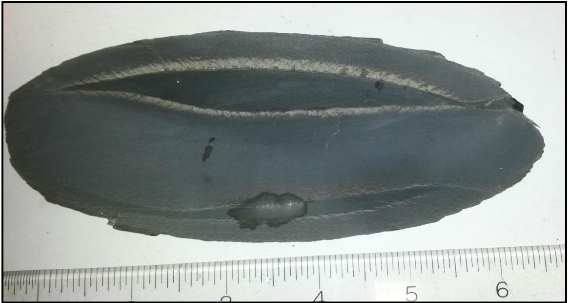
Cross section of smooth concretion showing two bands of cone in cones structures, slight epoxy infiltration in smaller band. Scale in inches.
