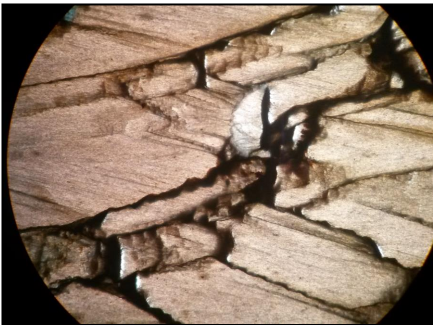
Cone shells, stylolites, annular rings, and carbonate cones in exterior crust (40x)
