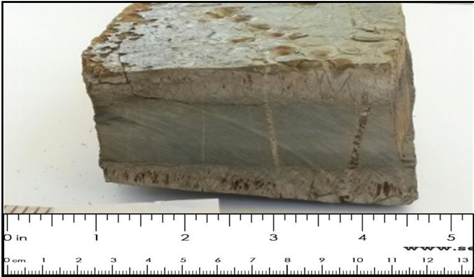
Side view exhibiting hydrothermal quartz veins cross cutting
