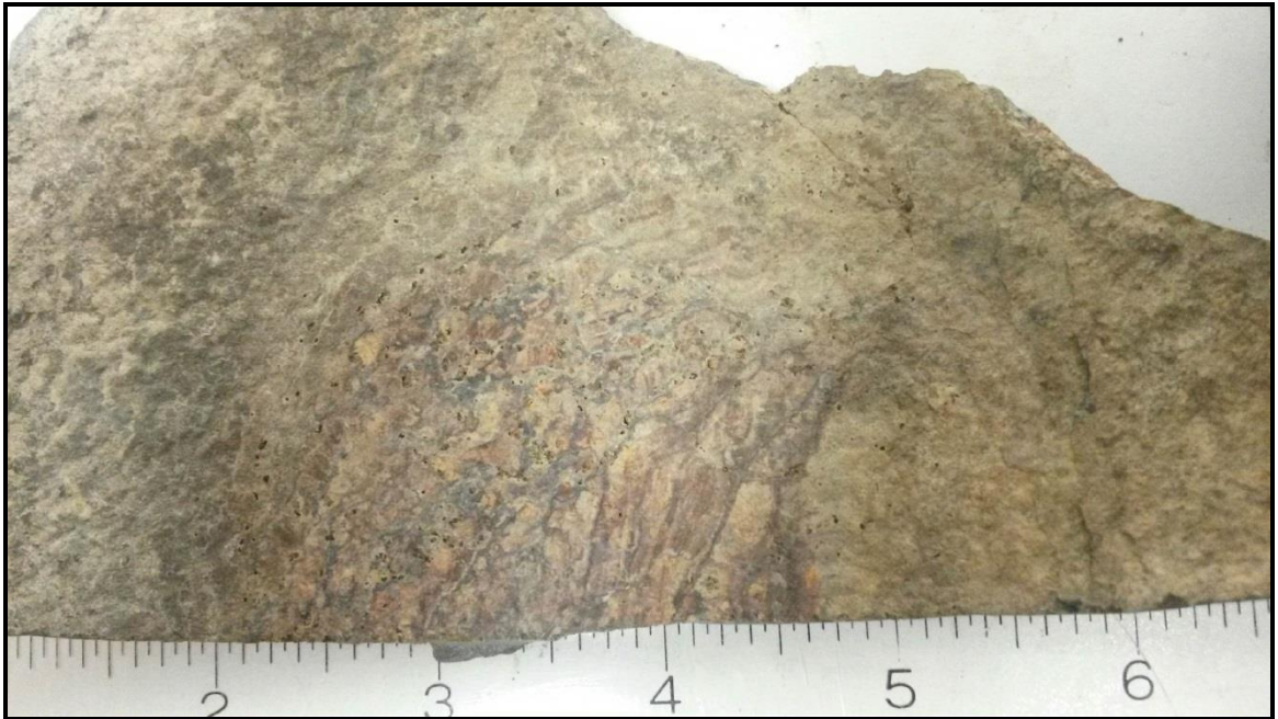
Iron staining on bounding surface near the cone structures with iron staining. Scale in inches.
