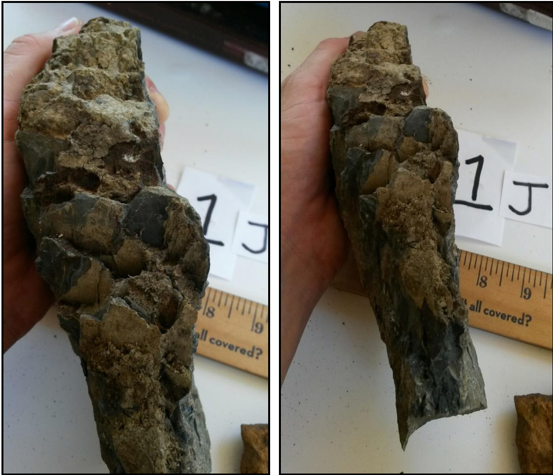
Top view exhibiting non-conformal surface crust. Scale in inches.
