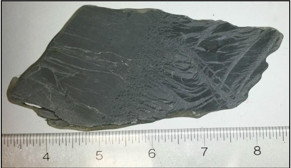
Cross section view with obvious slanted cones on one end with the small cone band in the middle. Visible exterior cones are on the left side without the fibrous “tentacle” precipitates. You would expect to see cone structures on the left side since they are present on the exterior. Scale is in inches.
