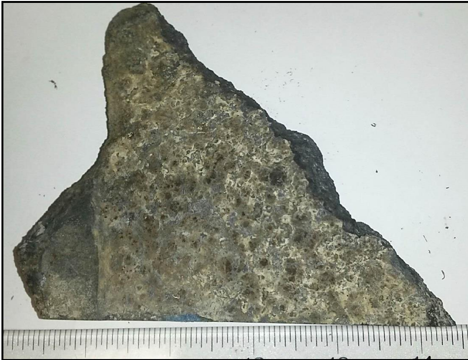
Bottom view exhibiting white crusty material and iron staining. Scale in inches.
