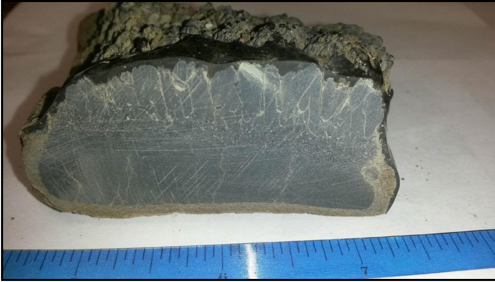
Cross section view showing upper and lower crustal differences and core. Epoxy is present on the top crust. Scale in inches.
