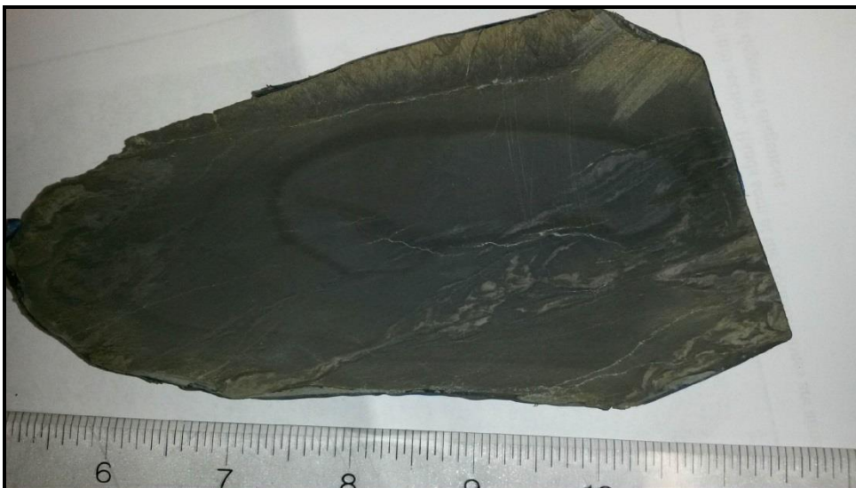
Cross sectional view showing cones at the top and lighter core area with halos present. Scale in inches.
