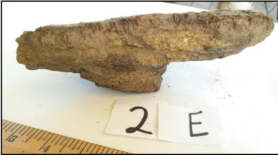
Side view showing multiple cone layers and variable core. Scale in inches.
