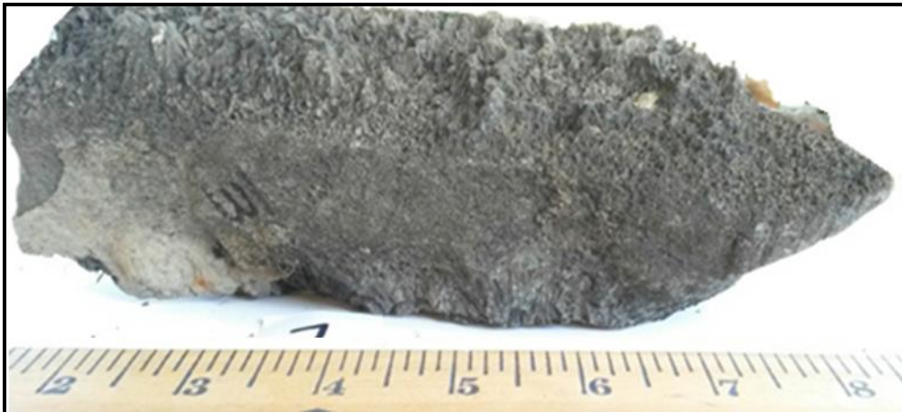
Cross section view showing granular core. Scale in inches.
